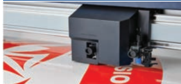
Powerful Cutting Head: 600gf
